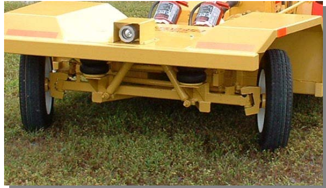
MAC-XP standard with SOFT RIDE Front suspension
