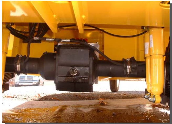
MAC-XP with double reduction rear end with enclosed wet brakes.
